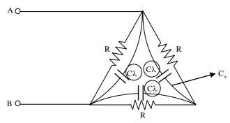
$Z_{\Delta} = 3Z^*$ , but in capacitor case  $Z = \frac{1}{j\omega C}$ , So if the capacitor of star network are C each
