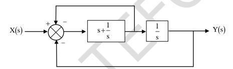
$$\frac{Y(s)}{X(s)} = \frac{\frac{\left(s^2 + 1\right)}{s} \times \frac{1}{s}}{1 + \frac{s^2 + 1}{s} + \frac{s^2 + 1}{s^2}} = \frac{\frac{\frac{\left(s^2 + 1\right)}{s^2}}{s^2 + \left(s^2 + 1\right)s + s^2 + 1}}{s^2}$$
