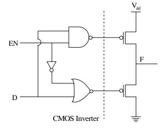
→ NAND gate enabled, when their enable input is "1" and NOR gate enabled, when their enable input is "0".
