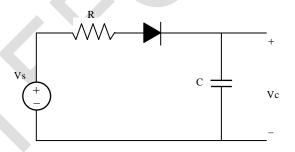
For positive half cycle, diode will be forward biased and capacitor start to charge
