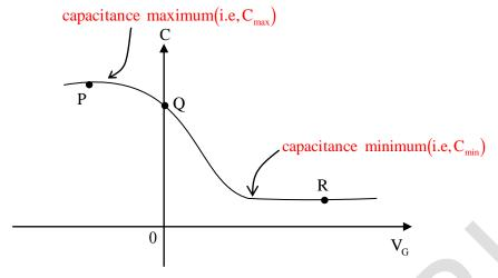
At higher frequency  $C_{\min}$  minimum capacitance obtained in inversion-regime so point R-belongs to inversion regime.
