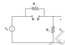
$$V_{L} = \frac{R_{2}}{R_{1} + R_{2}}.V_{S} = \frac{50}{100} \times 8V = 4V$$
