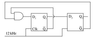
$$\begin{array}{c|ccccc} D_{2}(Q_{1}) & D_{1}(\overline{Q}_{1}.\overline{Q}_{2}) & Q_{2} & Q_{1} \\ \hline - & - & 0 & 0 \\ 0 & 1 & 0 & 1 \\ 1 & 0 & 1 & 0 \\ 0 & 0 & 0 & 0 \end{array} \xrightarrow{f^{st} \ clock} \begin{array}{c|cccc} Initially \\ 2^{rd} \ clock \\ 3^{rd} \ clock \end{array}$$
