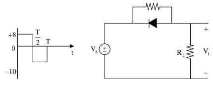
Case (i) For +ve half cycle diode is reverse bias:
